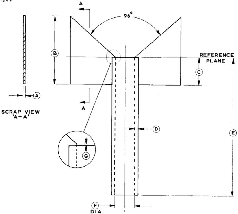
The gauge shown above will pass freely over base and neck to the reference line, and when rotated through 360° the blades of the gauge will contact the flared neck at the reference line only.
